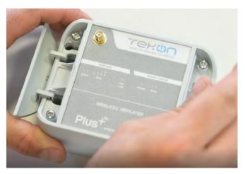
**02** Connect a micro USB cable to the computer and then to *WRP001 PLUS Wireless Repeater*.
