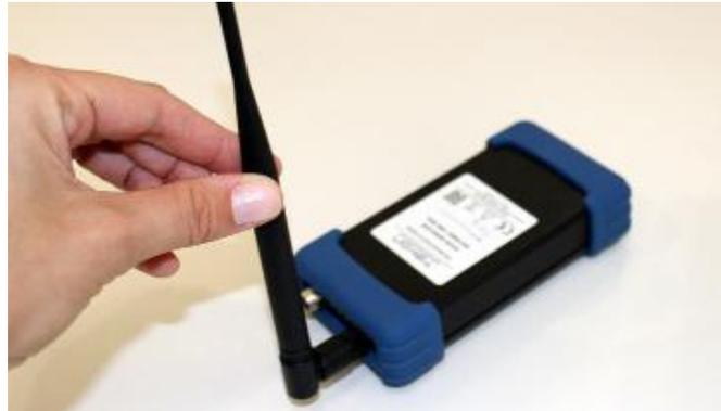
**02** Connect the *DUOS RS485-USB* cable to the computer and then to the Gateway.
