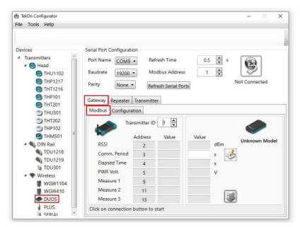
Ensure that the Port name, Baudrate, Parity and the Modbus Address fields are the same obtained in configuration mode.
