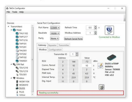
The messages *Connected to Modbus* and *Reading successfully* will appear if the *Serial Port* configuration parameters are correct and the Modbus connection established.
