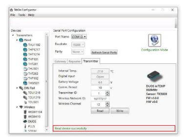
The status string at the bottom of the software window gives feedback on reading operations.
