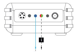
LED switches on and remains steady
