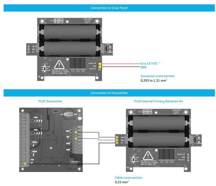
Note: If "PV" connection is in use, PLUS wireless transmitter will send battery voltage to gateway, otherwise the transmitter will provide "Power Out" voltage.
