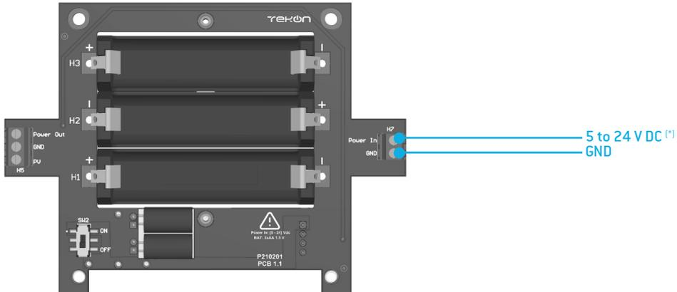
(\*) External power can work simultaneously with primary batteries. Batteries work as a backup power when external voltage is equal or higher than 5,5 V.
