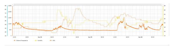
Graphic created on the IoT platform by collecting temperature, humidity and CO2
