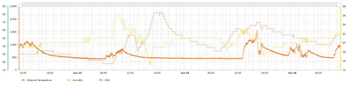
Graphic created on the IoT platform by collecting temperature, humidity and CO2
