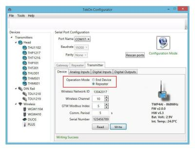
Figure 1 - Tekon Configurator window with the TWP4AI transmitter double configuration
