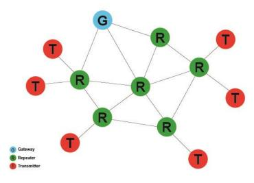
Figure 2 - Mesh network typology
