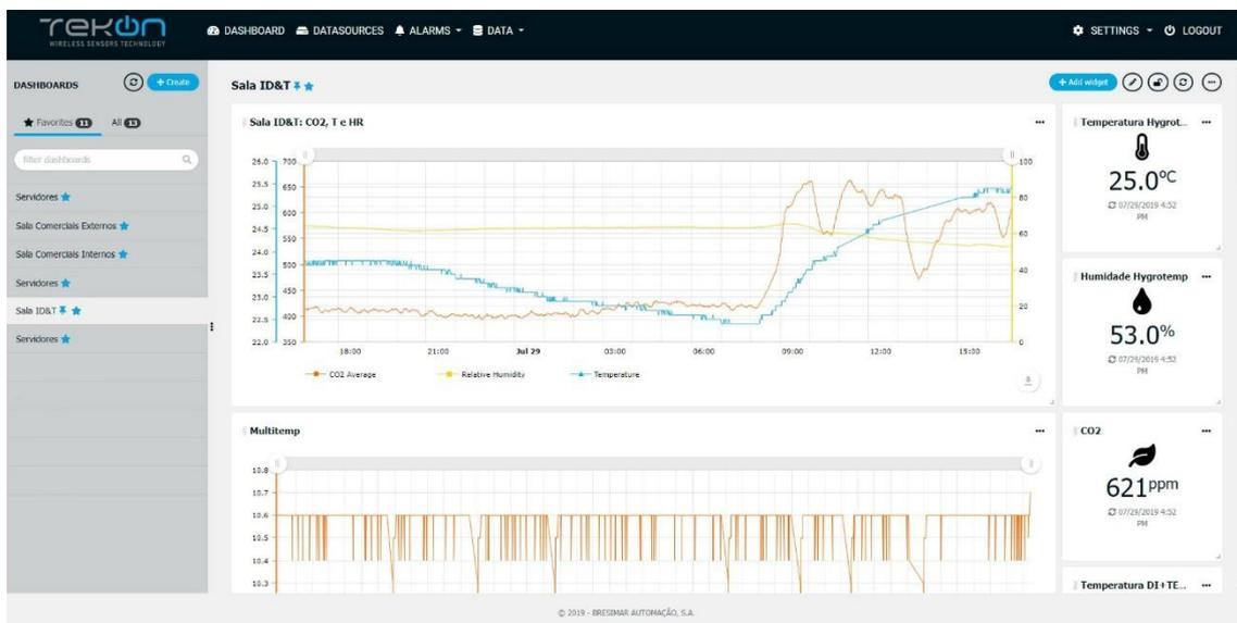
Figure 2 - Graphical example of readings on Tekon IoT Platform
