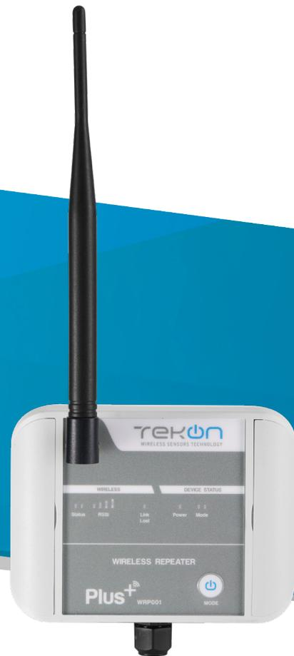
PLUS WRP001 Wireless Repeater provides extra communication range by supporting up to 13 hops (12 repeaters in series).
