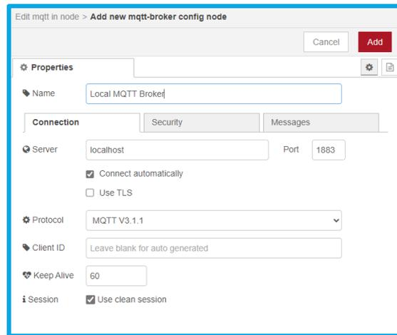
Figure 156 - MQTT Server configurations.
