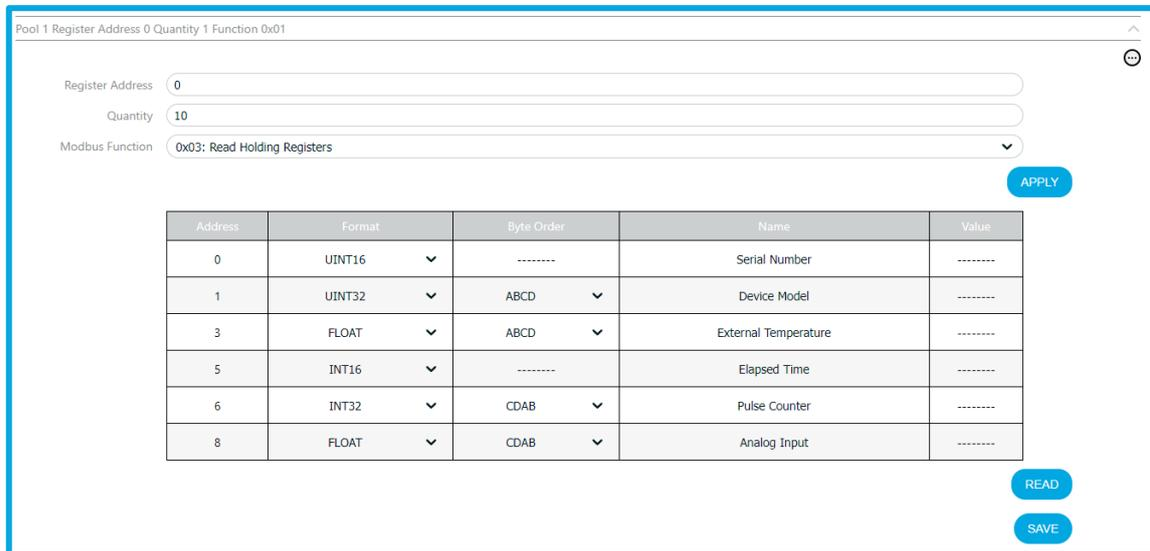
Figure 135 - Modbus RTU window section to configure Modbus RTU addressing.
