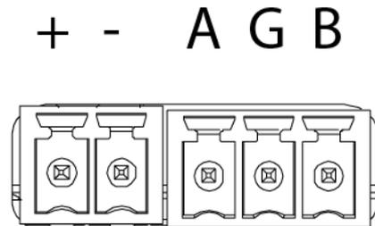
Figure 8 - Power and RS485 connections (aluminum case)
