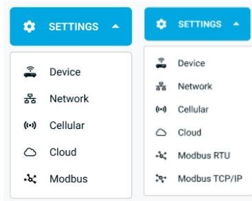
Figure 99 - Settings tab menu with the Modbus RTU Master and TCP/IP Client Pack inactive (left) and active (right).
