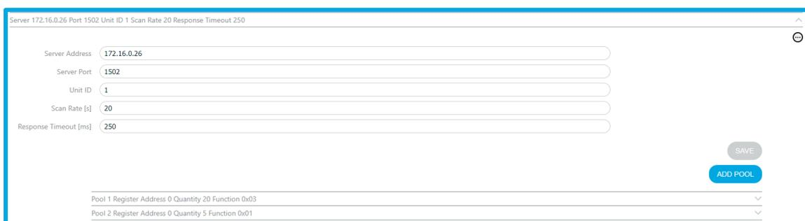
Figure 140 - Modbus TCP/IP window section to configure server requests.
