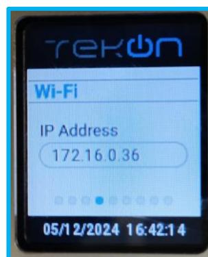
Figure 118 - uGateway display showing the Wi-Fi connection IP.
