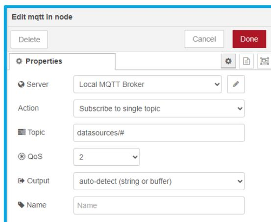
Figure 158 - MQTT Node configuration.
