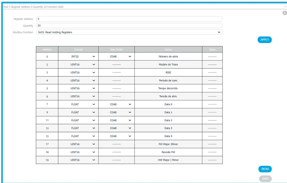
Figure 139 - Modbus TCP/IP window section to configure Modbus TCP/IP addressing.
