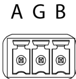
Figure 7 - RS485 connections (ABS case)
