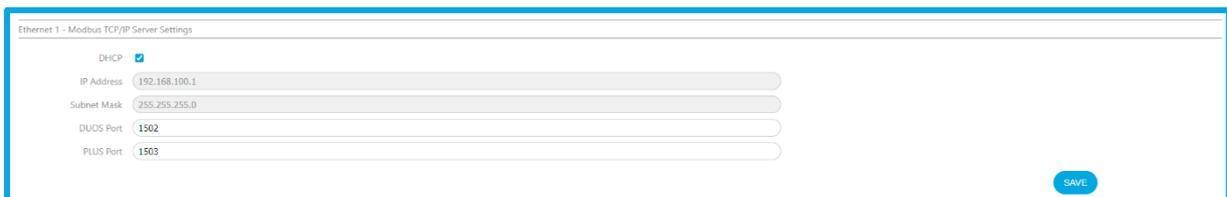
Figure 132 – Modbus TCP/IP section on the Modbus Settings page in the base version of the device.
