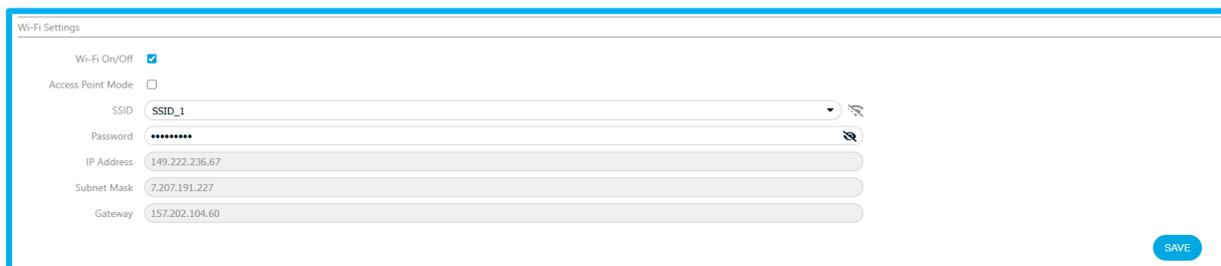
Figure 116 - Fields to be filled in to connect to a Wi-Fi network.
