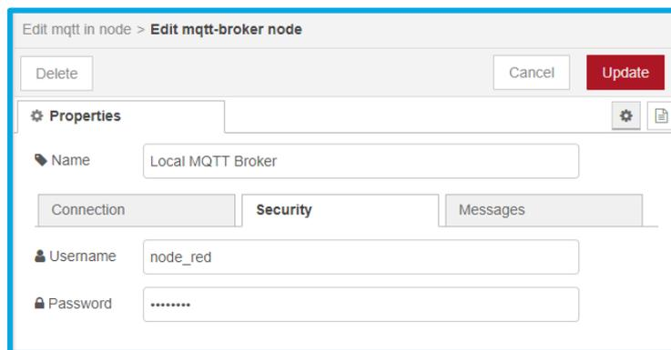
Figure 157 - MQTT Server configurations.
