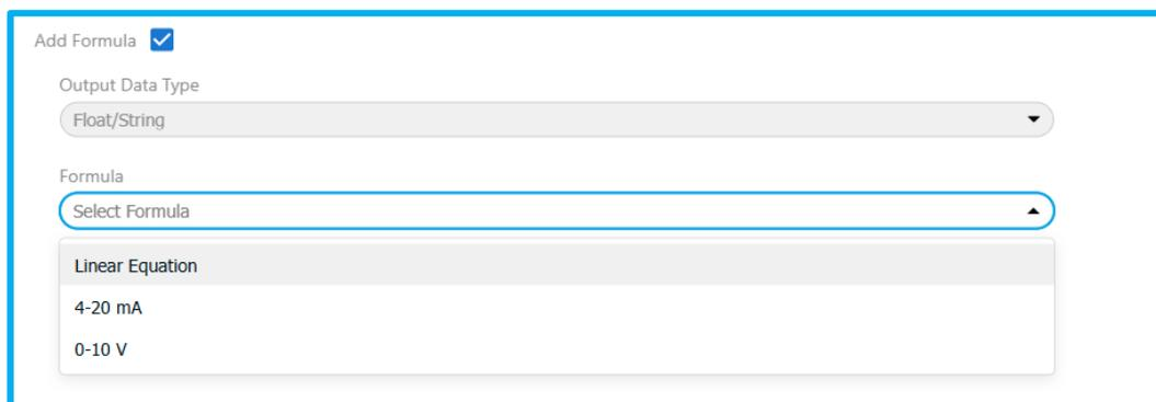
Figure 67 - Formulas for float-type data outputs.
