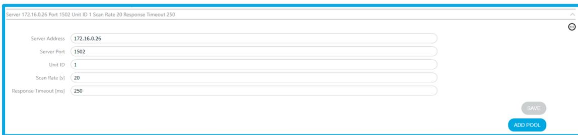
Figure 138 - Modbus TCP/IP window section to configure the server.
