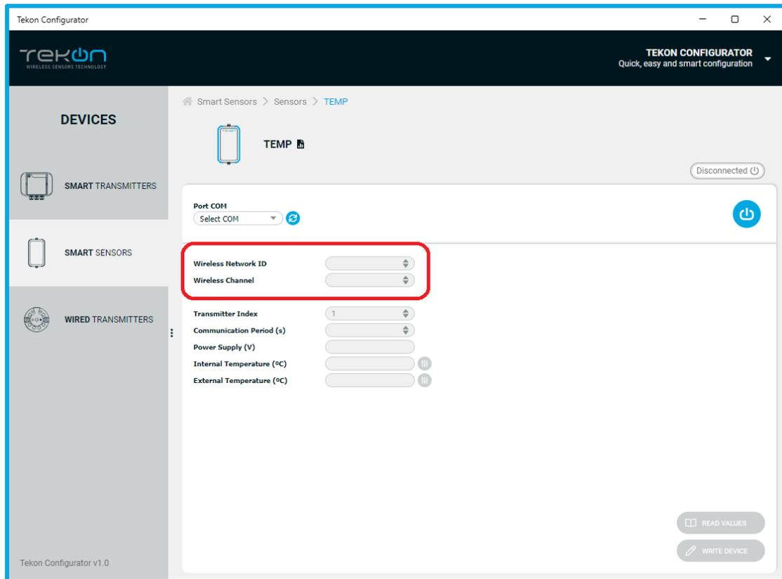
Figure 58 – Transmitter configuration page in the Tekon Configurator.
