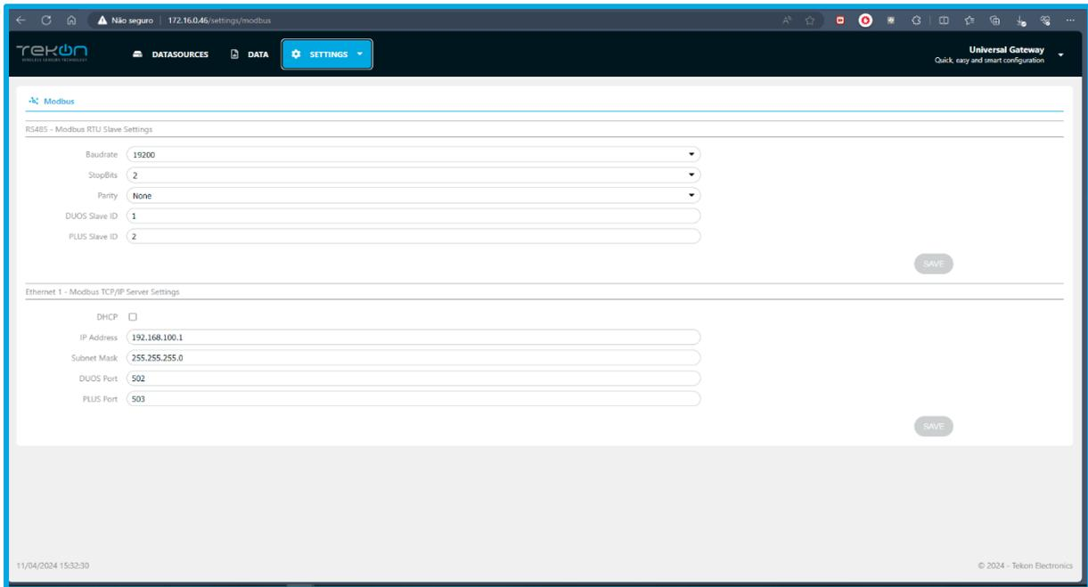
Figure 130 – Modbus Settings page in the base version of the device.
