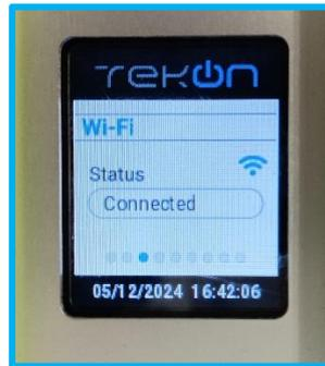
Figure 117 - uGateway display showing the Wi-Fi connection status.
