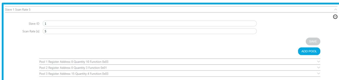
Figure 136 – Modbus RTU window section for configuring slave requests.
