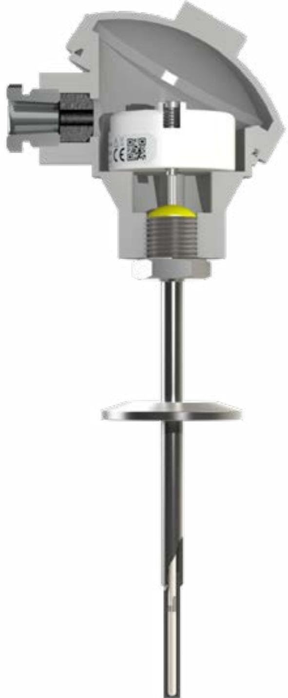
These types of sensors are based on the principle of variation of electric resistance according to the temperature. The most used materials for the manufacture of this type of sensor are platinum, copper or nickel. Metals with the following features:
