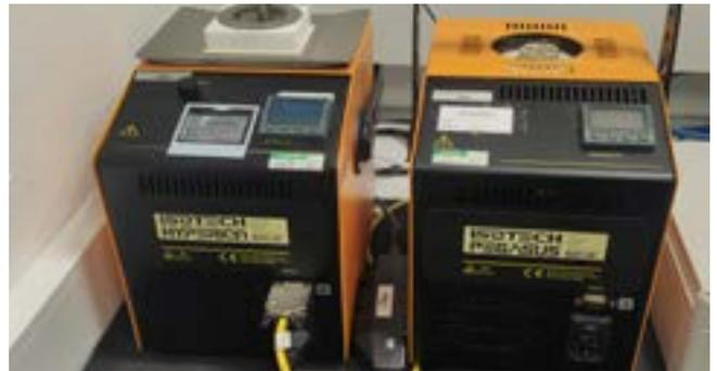
Dry and oil bath furnaces are high-precision and stability equipment used for validations and internal characterizations.
