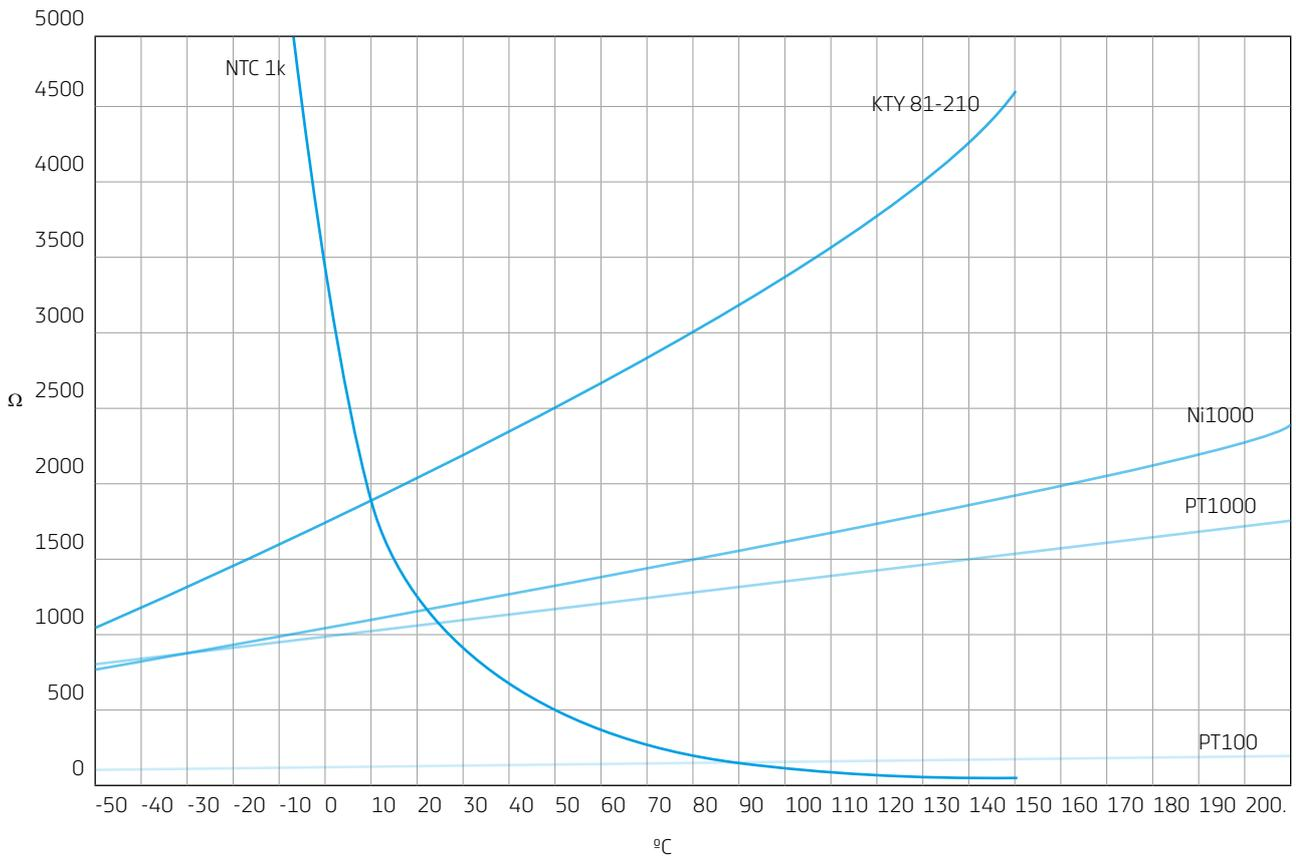
**Advantages and Disadvantages between the various temperature sensors (RTD)**
