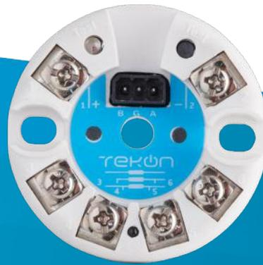
Tekon Electronics In Head Temperature Transmitters are specifically designed to meet the most rigorous requirements of operation in the industrial process environments. Due to their reduced dimensions they can be installed in the the DIN Form B sensor connection head in place of traditional terminal blocks.
