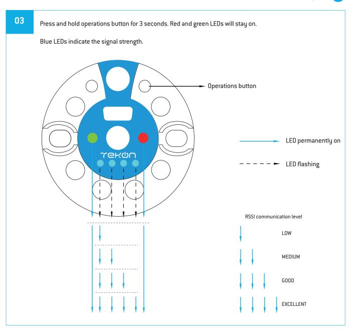
Press and hold operations button for 3 seconds to exit Site Survey Mode and activate normal operation mode.
