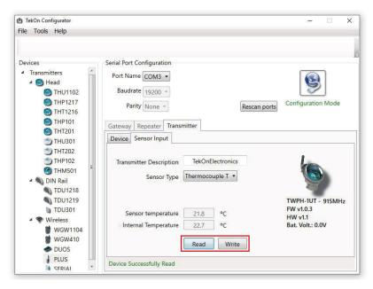
Click on Configuration Mode ( ) button to exit from configuration mode to normal operating mode.
