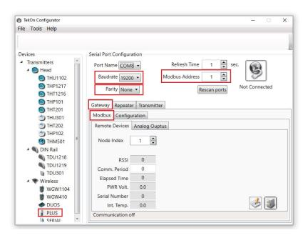
Ensure that *Port name*, *Baudrate*, *Parity* and *Modbus Address* fields are the same as those obtained in configuration mode.
