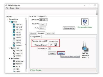
OB Click on Configuration Mode () button to exit setup and resume normal operating mode.
