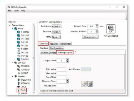
Considering the transmitter configuration with GTW Modbus Index=1, there is a Gateway Modbus Address Window corresponding to Modbus address window [0-19].
