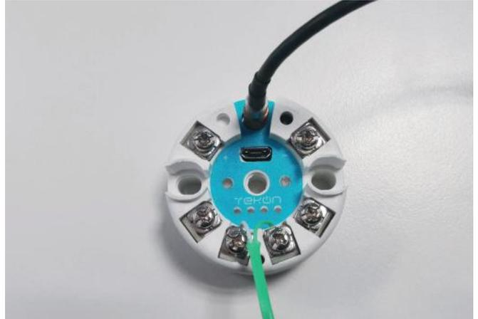
**02** Connect the micro USB cable to the computer and then to *TWPH-1UT PLUS Wireless Transmitter*.
