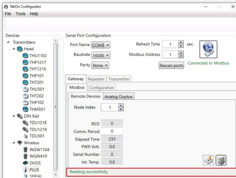
The messages *Connected to Modbus* and *Reading successfully* will appear if *Serial Port* configuration parameters are correct and the Modbus connection is established.
