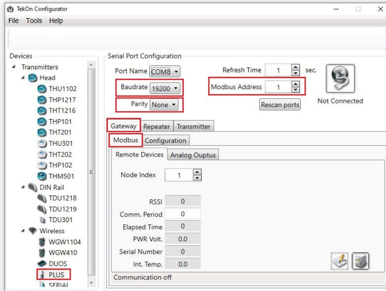
Ensure that *Port name*, *Baudrate*, *Parity* and *Modbus Address* fields are the same as those obtained in configuration mode.
