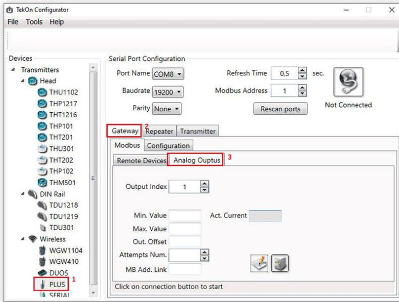
**03** Considering the transmitter configuration with GTW Modbus Index=1, there is a Gateway Modbus Address Window corresponding to Modbus address window [0-19].
