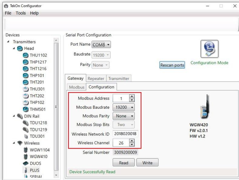
**NOTE:** The wireless network connection between devices is ensured by setting the same *Wireless Network ID* and *Wireless Channel* parameters.
