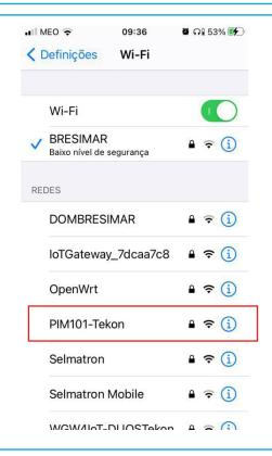
PLUS PIM101 IoT has a fixed IP address assigned to be accessed via mobile phone, tablet or pc (through Wi-Fi). The interface designed to interact with the device can be accessed through its fixed IP (192.168.128.1) or its SSID address (http://Tekon). The factory-defined and configurable access data:
